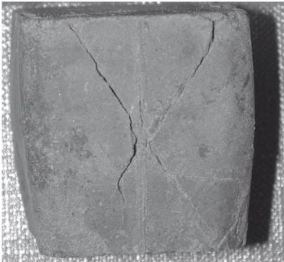
Fig. 3. Formation of slip lines along directions of maximum shear stress during uniaxial compression, which leads to crack opening at larger strains.
