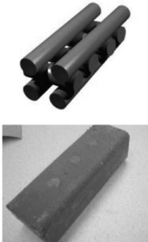
Fig. 6. (a) Generic bi-directional fibre lay-up for tensile/compressive and compressive loadings. (b) Example of bittersweet chocolate reinforced with Super Nibs ® fibres.
