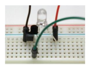
Arrange the LED and two transistors in the arrangement pictured in the above schematic and breadboard picture. Be sure to reference the transistor info sheet which will tell you how the schematic image of a transistor on the left relates to the transistor components on the right
