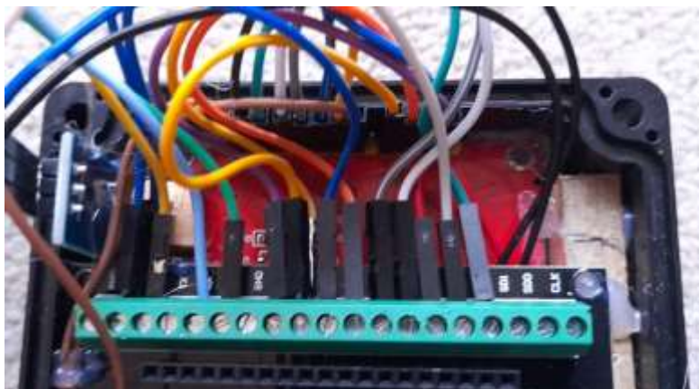
Buttons & encoder wiring. Note the choc-bloc to combine the GND wires and the piezo sounder.
