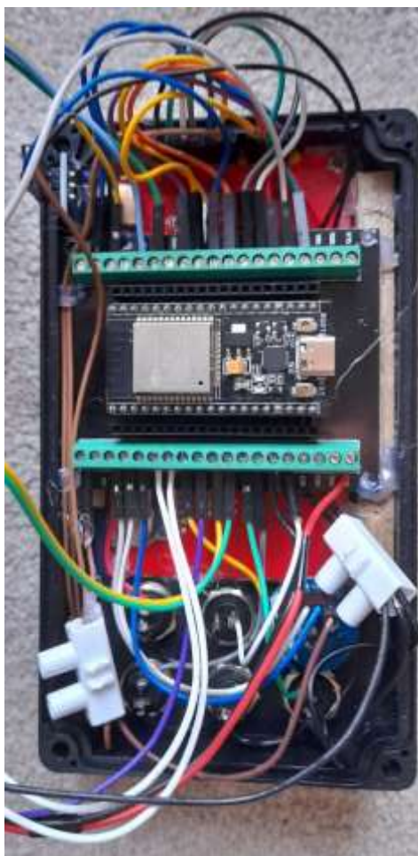
Buttons & encoder wiring. Note the choc-bloc to combine the GND wires and the piezo sounder.
