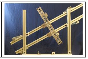
This is where the L brackets from the last two steps come into play. With the power supplies facing you, slide the four brackets on the back of the arms so that the top bracket is on the right and the bottom L bracket is on the left of the leg. Move these brackets until you are comfortable with the angle of the guitar.
