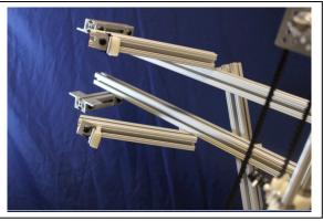
These foam blocks attach to the loose L bracket on the end of the arms located just above and below the strumming assembly. Thread one end of each zip tie in a block through the hole of the L bracket. Close, tighten, and trim the zip ties. Repeat for each foam block and bracket.
