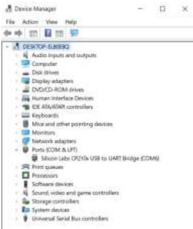
If the driver is missing, as shown on the screen below **(Yellow Triangle)** refer to the document Installing CP2102 Driver. Found in the github repository.
