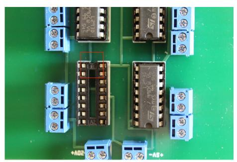
The red box shows the "16" on the socket facing the gap in the white.
