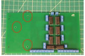
Line up the Arduino with the bottom two holes. Use it to mark these three holes, as there are only 3 holes on the Arduino that can fit M3 bolts. Pre-drill the holes with a 5/64 bit, then drill with a 9/64 bit.
