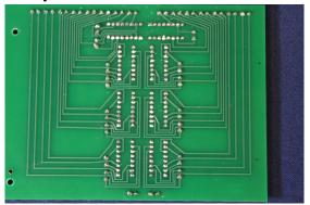
Holding your PCB up to the four L Brackets it must attach to, mark the spots on your PCB to drill.
