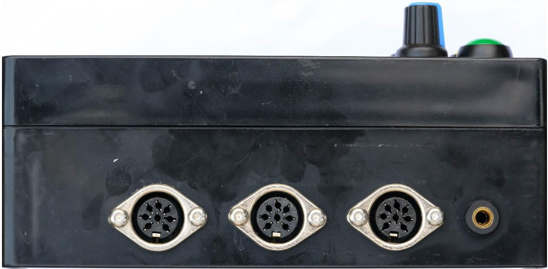
Side of box with sockets fitted.
