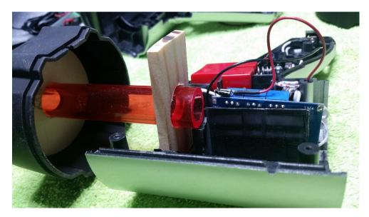
Step #12 Wire the laser module-
