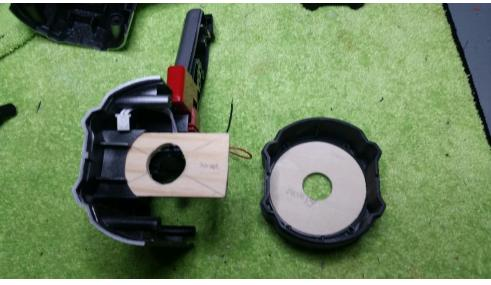
Test fit the plexiglass tube through both wood supports. There should be no wobble. I also painted the disk side facing outward red to match the plexiglass tube.
