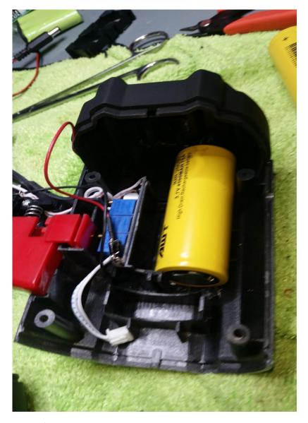
Test for clearance by snapping together both halves of the housing and the end cap.
