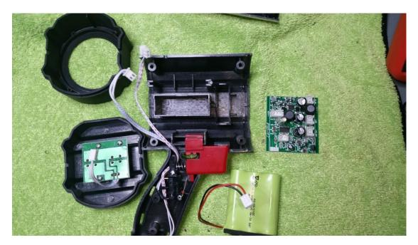
Make sure to remove the trigger-hold piece shown below. Just wiggle it out. It will not be included in the final assembly.
