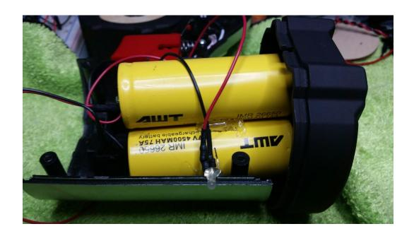
If you need to snap together the other half of the housing to convince yourself the fit is correct then do so. Use some hot glut to secure the LED in place. Once the glue dries insert the power supply plug into the flashlight power jack located in the base of the handle. The LED should turn on. Now unplug power to the power jack so the LED turns off.
