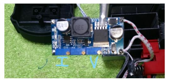
Next adjust the voltage limit by attaching a voltmeter across TP1 and TP2. The potentiometer on the far right (shown above) is use to adjust the voltage. Turn
