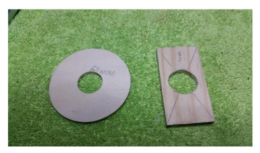
When creating these parts adhere closely to the outside dimensions so that both pieces fit snug into the flashlight housing.
