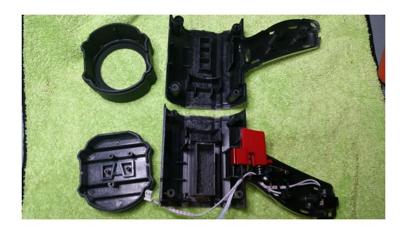
Step #5 Creating a cavity for the batteries-
