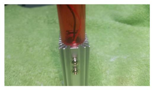
Now with your glue gun tack two places at the intersection of the tube and heatsink with a small amount of glue. Fine adjust the heatsink to make sure it's centered on the tube, make haste before the glue sets. If you mess up the alignment just remove the two small tacks of glue and start again.
