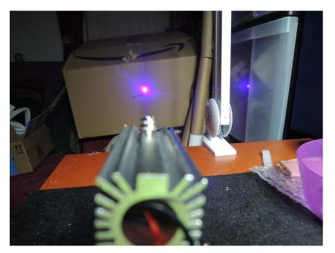
Once the focus is set remove power from the laser. Remove the laser module from the heatsink. Apply a very thin coating of heat conductive grease to the module then insert it back into the heatsink as shown below. This is the reverse of that used to adjust the focus pictured above. I chose this orientation because it protects the lens from dust and the focus ring from being bumped and going out of focus. Tighten the screws just firm.
