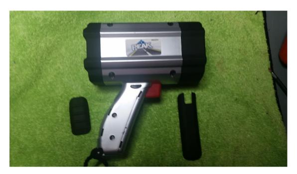
Now remove the (6) screws, with a little giggling the housing separates into four pieces. Be careful here because the trigger is spring loaded and it needs to be kept intact with the housing.
