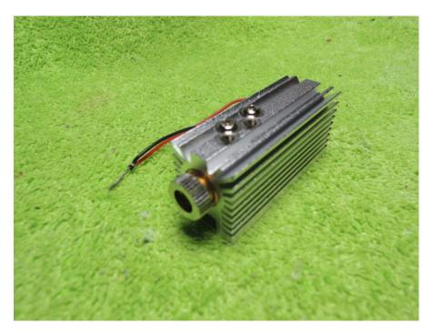
To set the focus use the power supply that comes with the flashlight to power the laser. I made a simple adapter to plug the power supply into then use alligator clips to connect to the laser module.
