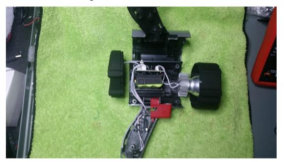
Remove the circuit board and unplug all connecting wires. Unscrew and remove the circuit board located in the end cap. Remove the (4) small screws from the lens head to remove the LED housing, washer and glass lens. Set aside the (4) small screws and washer for reuse later. Only the trigger, and power jack in the handle will remain. This flashlight includes a power supply that will be used to charge the internal battery. Keep the other internals for your next DIY project!
