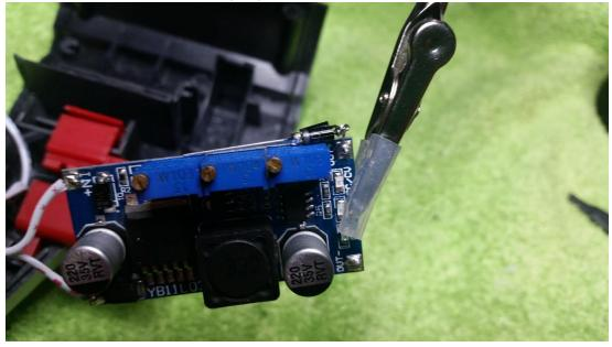
The charger board can be test fitted in the cavity already provided by the existing housing. As it just happens, it fits perfectly without any modifications.
