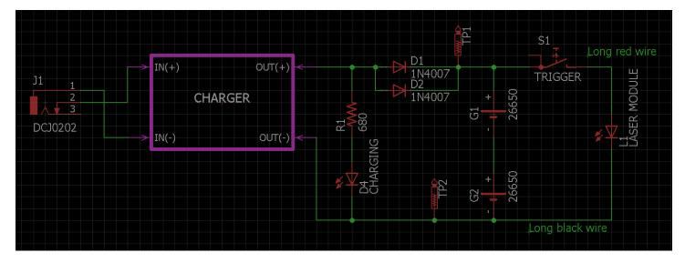
Cut off the white connector leading to the power jack then solder the wires to the IN(+) and IN(-) pads of the charger board as shown below on the left side. The two white wires are labeled with "+" and "-". Double check to make sure you get this correct.
