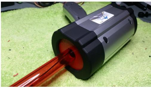
If you were precise in making your wood support pieces the tube should be fairly rigid. I added a bead of hot-glue around the tube where it passes through the rectangular support piece hole. This will prevent the tube from sliding out of the housing. I did not apply glue to the disk because if disassembly is necessary the head piece will slide down the tube away from the housing.
