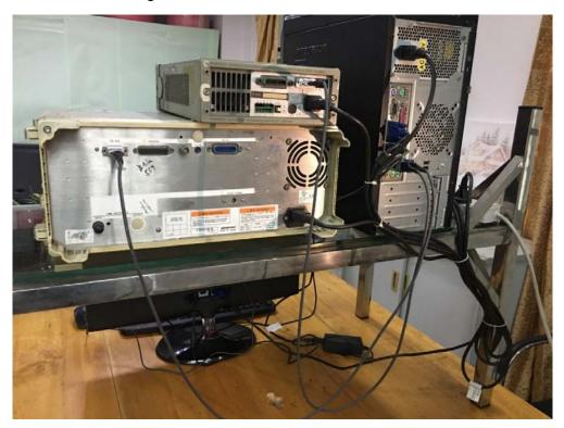
The above devices are connected to the PC through the RS-232 interface since the PC doesn't have a physical serial port, we need to use a USB to RS-232 converter for instrument connection.
