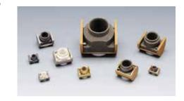
Rivetless nutplates eliminate the need to retain nutplates with rivets, thus reducing weight and manufacturing costs. There is an added benefit of increased fatigue performance since the stress concentration associated with the rivet holes is eliminated. One design, the Simfast™ rivetless nutplate, is a multi-piece fastener that incorporates a replaceable nut element, and is used in both engine and airframe applications.
