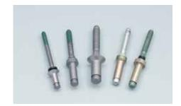
The Ergo-Tech® blind fastening system is designed for both metallic and composite structures. It is available in shear and tension head configurations. Its corebolt breaks flush with the top of the sleeve every time. The one-piece sleeve configuration and no threads in bearing result in high structural integrity and high-retained clamp-up. Lightweight ergonomic tools are available to install the system. The Ergo-Tech® fastener is also ideal for robotic installation.
