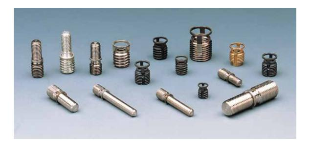
Kelox® inserts and studs are highperformance threaded products that typically require smaller diameter installation holes than other solid bushing inserts and studs. This translates into overall reduced boss sizes and weight savings. The Kelox® fasteners incorporate a pair of self-broaching keys joined by an integral ring that facilitates the driving of the keys into the structure.
