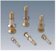
to develop an interference fit without composite delamination, and provides the grounding needed through the structure. With a titanium pin and titanium collar, the Flite-Tite® system provides high performance with the lowest possible weight.
