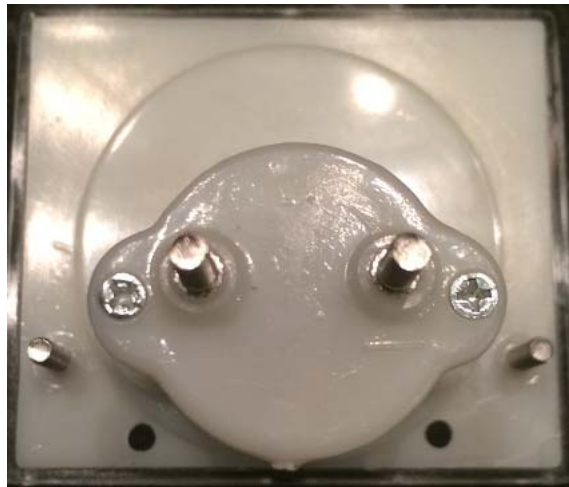
Figure 5.101 – Rear of meter with LED mounting holes
