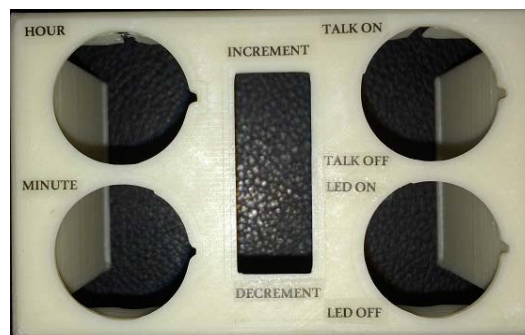
Figure 5.121 – Pushbutton Panel Labeling
