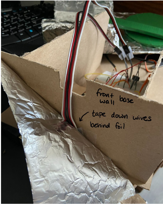
Figure 7: Ultrasonic Sensor Wire Taped Down
