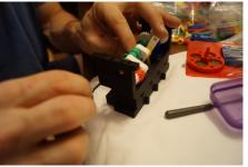
Now we need to adjust the length of the little rods extending from the Pistons. Turn your shafts so that one of your Piston rods is at its lowest point. Cut it off so that it is level with the Engine Block. Repeat this for the remaining 3 piston rods.
