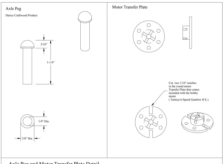
Axle Peg and Motor Transfer Plate Detail
