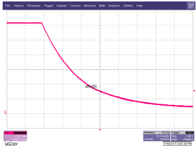
Figure 17. Gate Voltage of CHG FETs While Opening
