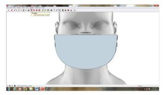
From the toolbar look for offset (two arcs with an arrow). Click on the surface to offset inwards. Input 400 mm and delete the center surface.
