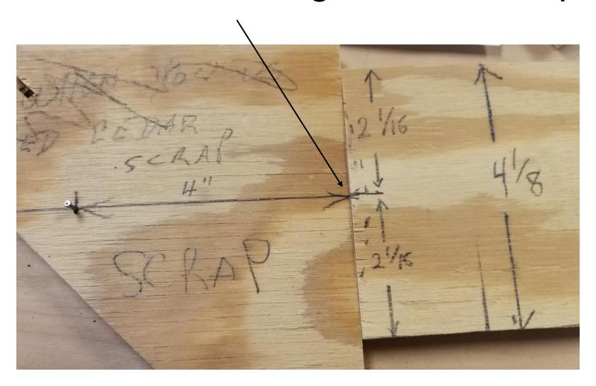
Hook the tape over the nail and rotate it. Mark the side piece at the 4-1/4" dimension of the tape. Short dashes are the easiest to mark.
