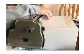
It is difficult to read and correct the braille "dots" as the paper comes out of the Braille Writer. This table provides support for the paper while reading and erasing. It is particularly useful when performing math calculations on the writer.
