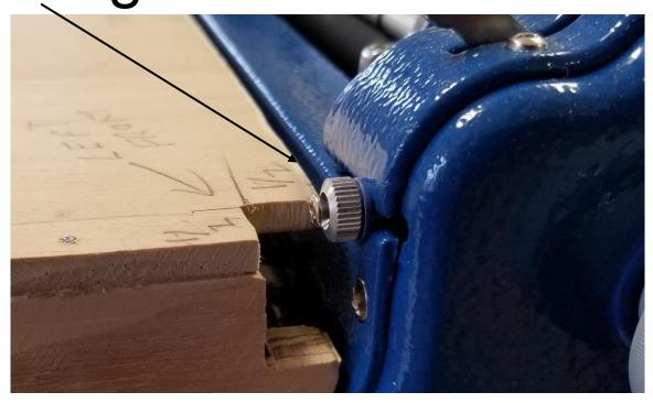
Sand off the bottom of the sides if needed to adjust the table height. Sand the center area of the sides to form "feet". The prevents rocking of the table.
