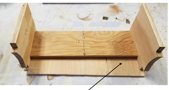
This inner support is too long. Lay it out as shown and mark the cut line. Now it fits between the sides.
