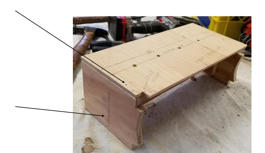
Test fit the table to a Brailler. The table top should be level or slightly below the Brailler discharge shelf
