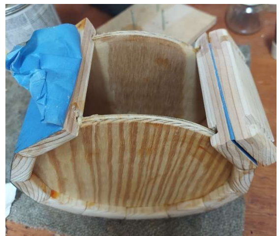
Figure 6- Stave channels being fitted to the Top and Bottom Panels
