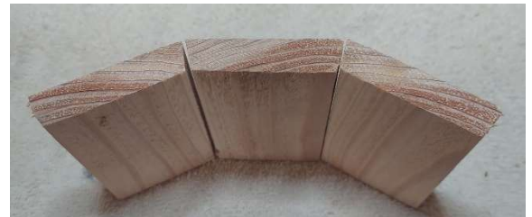
Figure 5- Stave segments cut at 15 degrees
