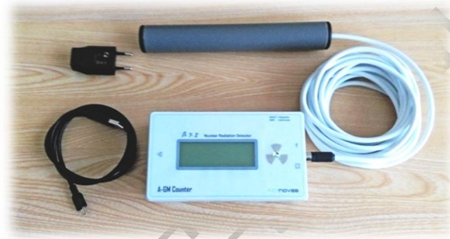
C-GM Counter with its external probe and power supply
