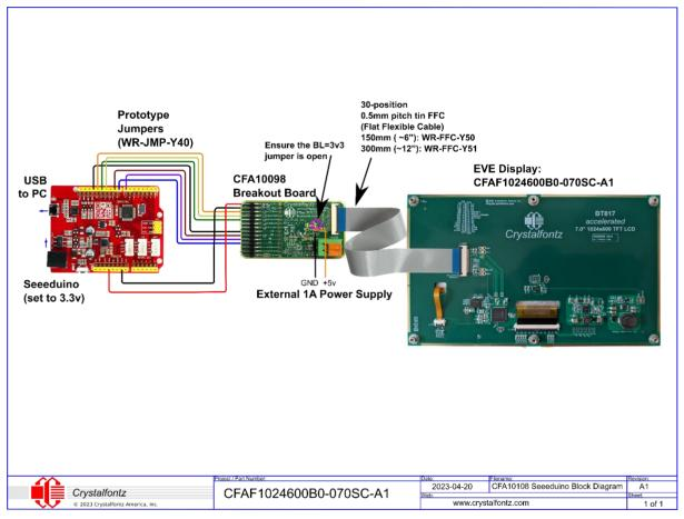
The CFAF1024600B0-070-A1-2 ships connected as shown (though the FFC may be disconnected to prevent breakages):
