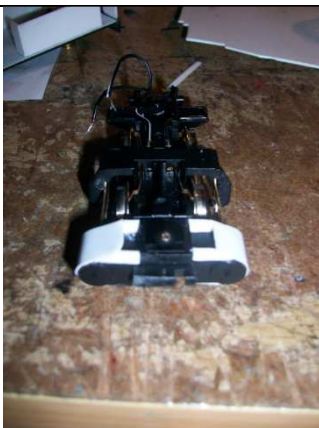
The frame work made up with plasticard, 30/000 with thinner card wrapped around, 10/000 was used for this.
