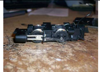
Cylinders there then glued to the chassis.
