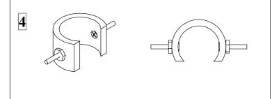
Apply a small amount of PVC cement on the inside of the screw head before inserting the screw in the hole. The glue will soften the plastic enough to allow the screw to sink into the pipe when the nut is tightened.
