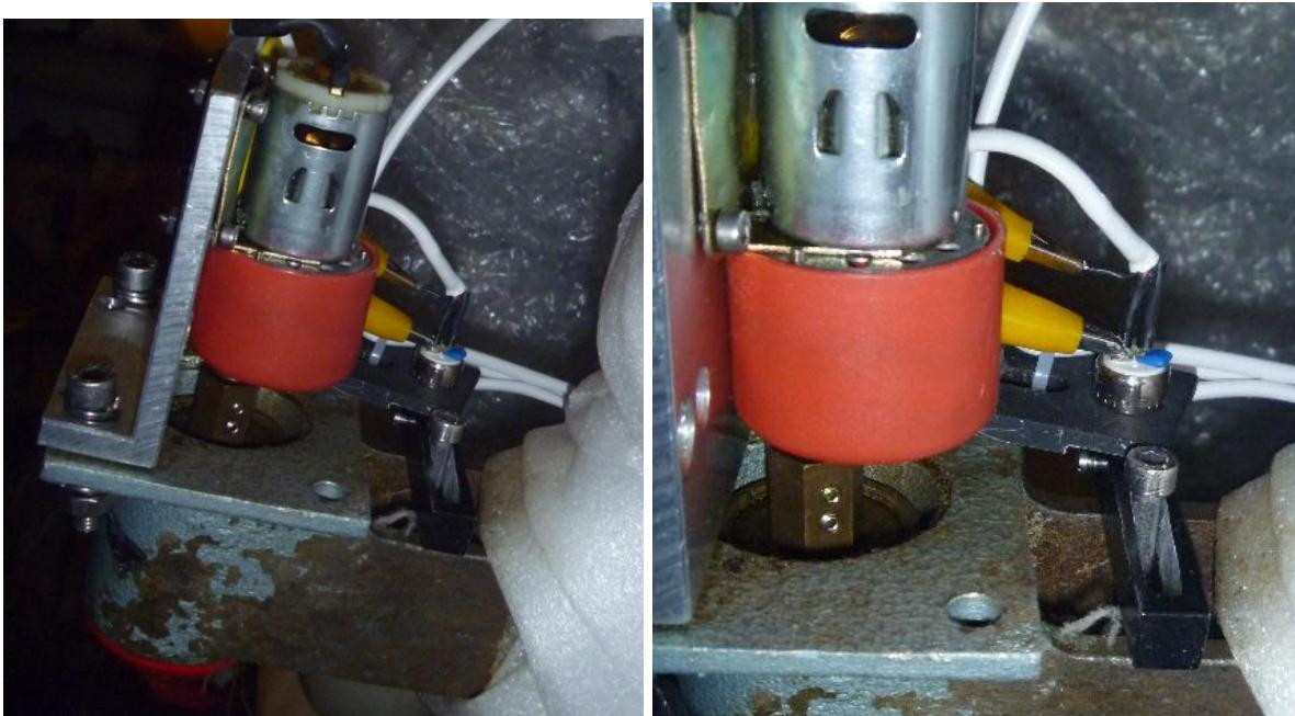
Speed 400 motor with 30 times redactor. From Conrad.de. Potentiometer 100 k with arm to sense how deep is valve.
