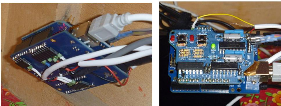
Extra connectors are soldered to Arduino. Motor shield is used.
