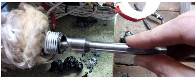
Using the screw to clean the barrel.
