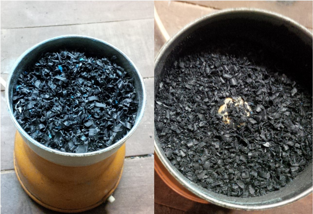
Coffee grinder before and after grinding for 30s to 1min. : Volume get divided by 2.
