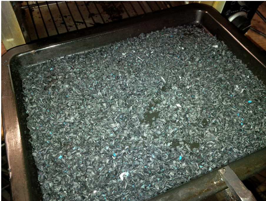
Plastic shavings entering the oven for drying. Blue and gray spots are some shavings from previous ABS grinding attempts.
