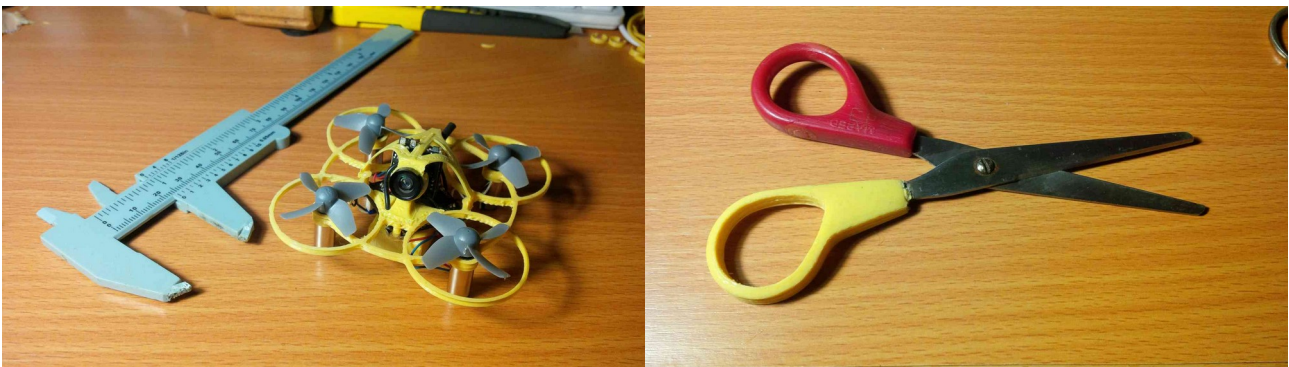
Early prints with recycled yellow PP filament : RC drone frame and scissors fix.
