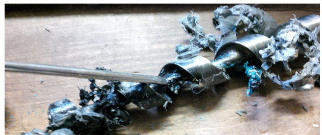
Removing sticky plastic with a screwdriver.
