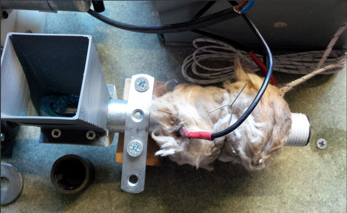
Extruder module with hopper, glass-wool isolated barrel, lead removed.
