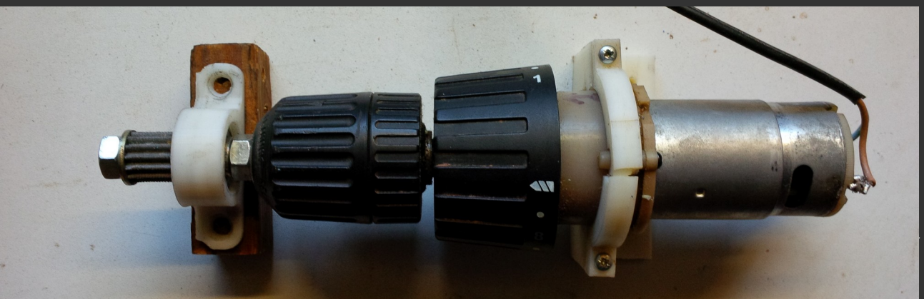
Cordless drill motor, gear box, overload clutch and chuck.
