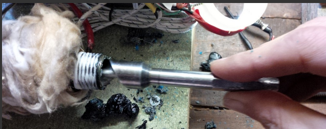
Using the screw to clean the barrel.
