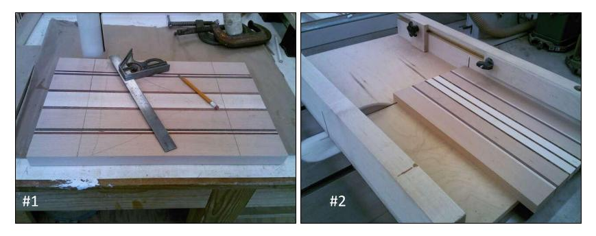
**Step #8:**Use an adjustable square and mark the desired length of the board. Photo #1.
