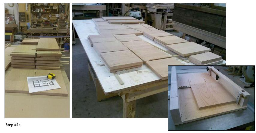
Cut the milled boards to length and width. The vertical boards are cut to 11" width. The horizontal shelves are 11 ½" wide.
