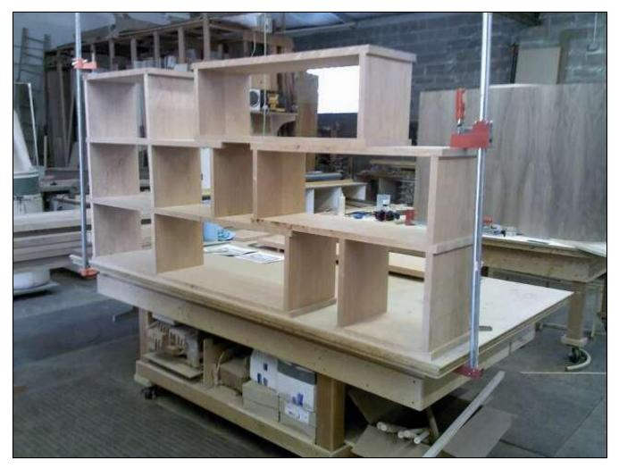
**Step #5:** Assemble and clamp the modules to ensure that they fit tightly. Make adjustments as necessary.
