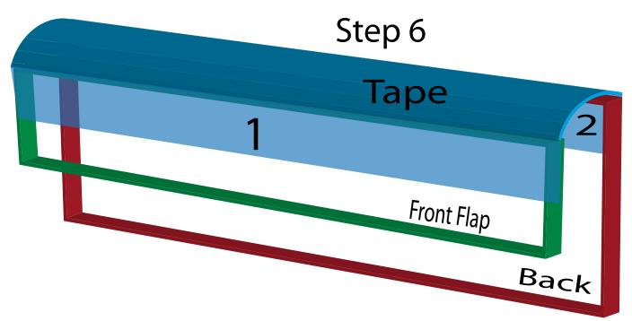
Place the front flap on top of the front Cover, Place tape on top of Front flap (1) then wrapping the tape the to back side(2), cut off any excess.
