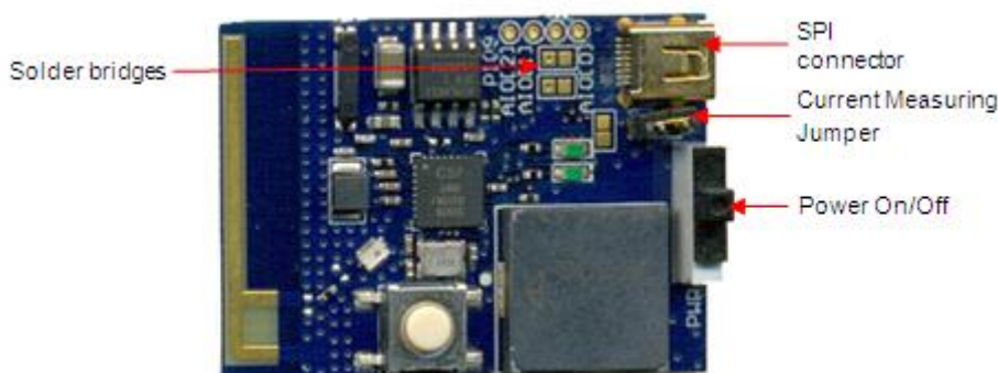
Figure 2.1: CSR1000 Development Board
