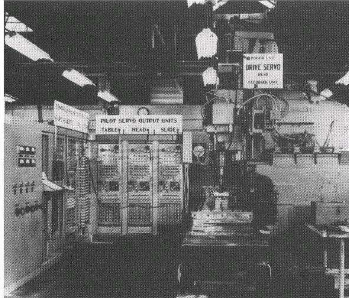
FIGURE 1-15 The first successful N/C machine, developed by MIT. (Courtesy of Cincinnati Milacron)
