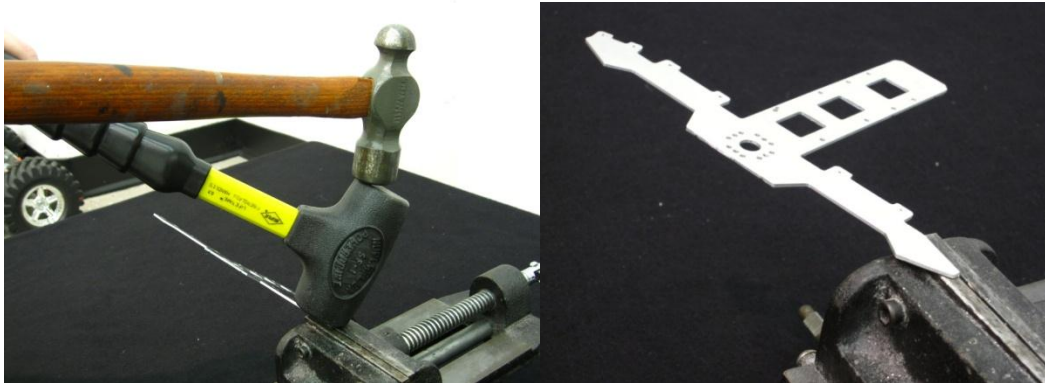
Figure 23: The mallet should make contact with the part in order to prevent scratches that may be caused by the impact of the hammer.
