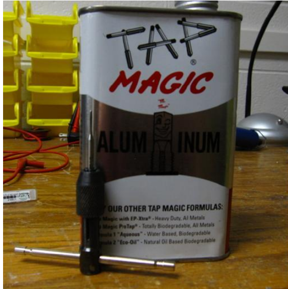
Figure 15: (Left) Tap handle after it has been attached to the appropriate tap bit. (Right) The result of a tapped hole.
