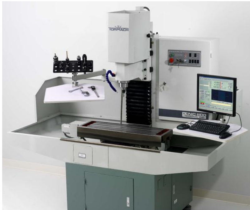
Figure 8: Tormach PCNC machine used in RoMeLa for the production of the DARwIn OP.
