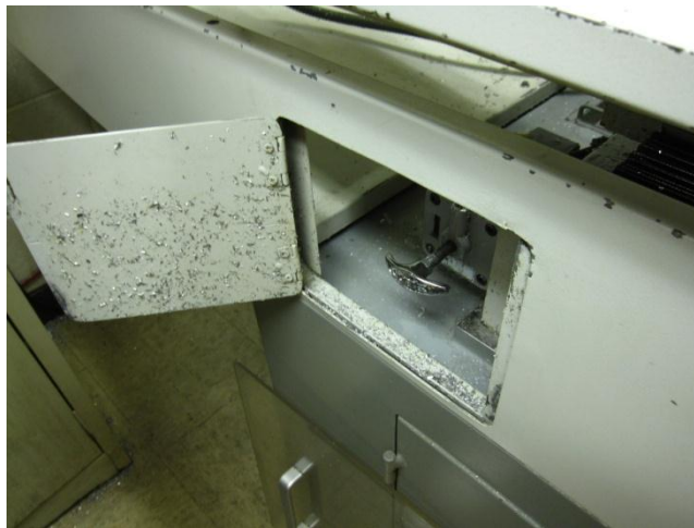
Figure 27: Pull the oiler to lubricate the ball screws on the CNC machine.
