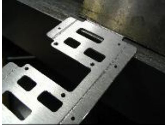
Figure 16: A properly clamped part. Notice the scoring line is still visible outside the clamp, and the edge of this line is aligned with the edge of the clamp.
