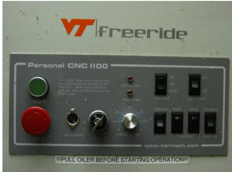
Figure 26: Control panel on the CNC machine. The button for spindle rotation is located at the bottom right corner.
