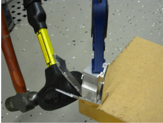
Figure 25: The mallet should make contact with the part in order to prevent scratches that may be caused by the impact of the hammer.
