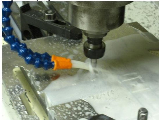
Figure 32: Make sure to have the coolant sprayed directly onto the tool to increase tool life.
