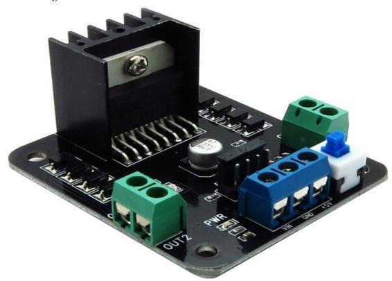
This module is based on the very popular L298 Dual H-Bridge Motor Driver Integrated Circuit. The circuit will allow you to easily and independently control two motors of up to 2A each in both directions. It is ideal for robotic applications and well suited for connection to a microcontroller requiring just a couple of control lines per motor. It can also be interfaced with simple manual switches, TTL logic gates, relays, etc.
