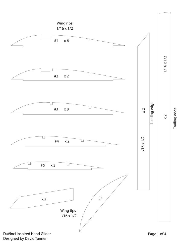
Glue this edge first Glue this edge second 1/16×1/16 1/16×1/16 Pin leading and trailing edges first 1/16 x 1/2 1/16 x 1/2 #2 rib  $1/8 \times 3/8$ rib
