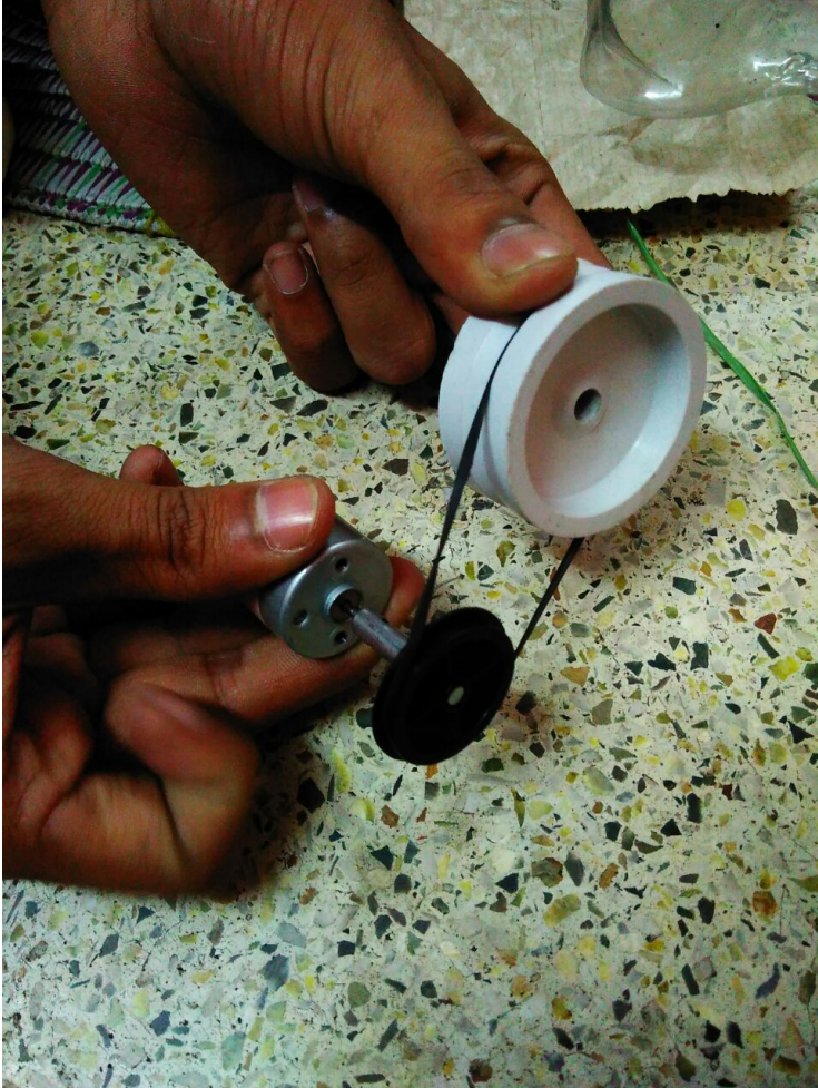
Figure 2: The pulley and the belt system connected to the shaft of dynamo
