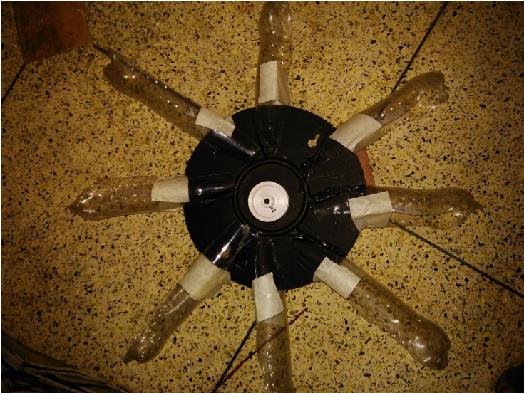
Figure 1: Runner with vanes made of Plastic bottles
