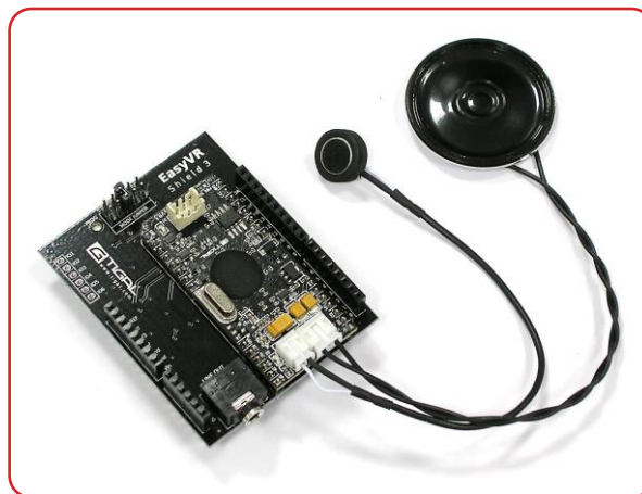
EasyVR Shield 3 fully assembled
