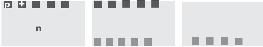
Figure 6. Side-view of a p on n diode structured to become a single-sided p on n [left], double-sided p on n [center] or a single-sided n on n [right] detector.
