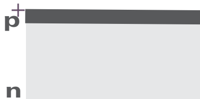
Figure 5. Side-view of a p on n diode. A typical detector is around 300\mu\text{m} thick. The p-implantation is around 1\mu\text{m} deep.
