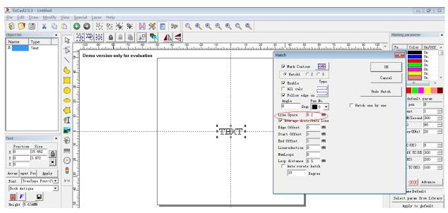
Normally you just need adjust line space, different line space will show different marking result, you could adjust from 0.01mm ~0.2mm, we recommend make it 0.05mm~0.1mm
