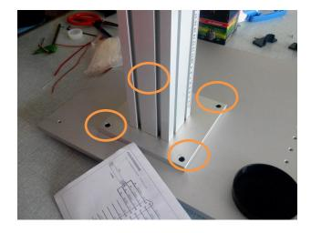
2.Install the laser tube, connect laser tube on the column, follow the
