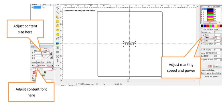
Tips: you could try different power( $0\sim100$ ) and speed ( $0\sim1500$ ), if you want deep marking, you could try high power and low speed, if you want mark fast, could adjust high speed.
