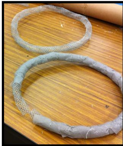
Figure 6: Airflow Tubes Under Construction
