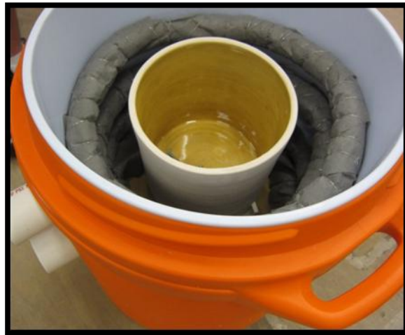
Figure 7: Airflow Tubes Surrounding Clay Pot
