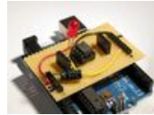
Stripboard Arduino shield for programming ATtiny45 and ATtiny85 by nikkipugh
