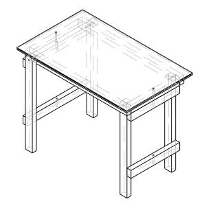
REQUIRED HARDWARE (NOT SHOWN): (2) 3/8" X 6"L CARRIAGE BOLT (4) 3/8" X 3.5"I CARRIAGE BOLT (4) 3/8" NUTS
