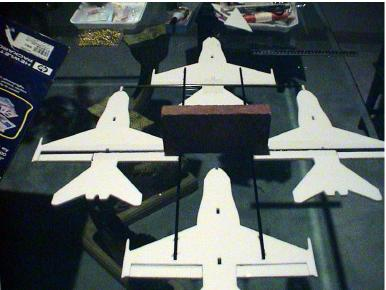
Piece of foam helps align the side planes keeping them square to the fore and aft shafts.
