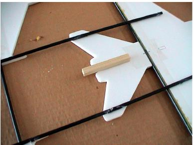
Tape servo wires down.
