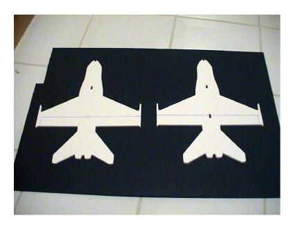
Cut out the ailerons and the tubing slot
