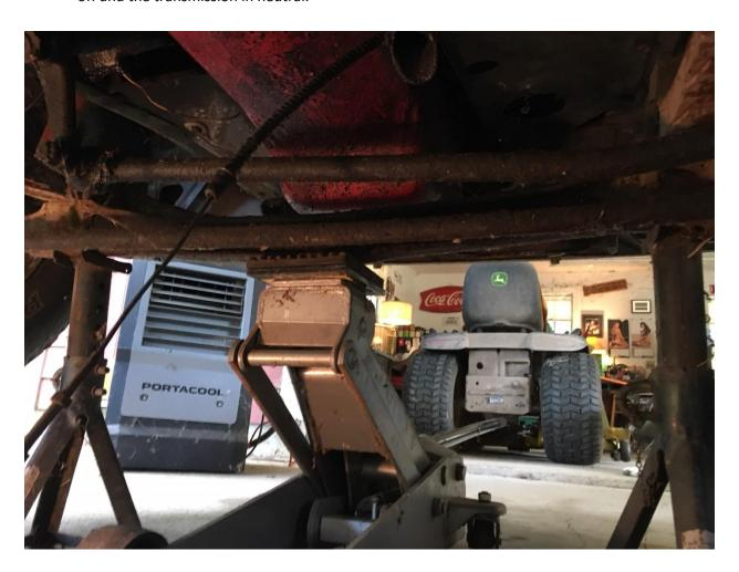
2. Disconnect the emergency brake cable at the brake lever past the transmission housing.
