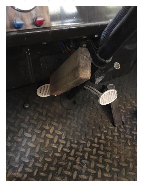
5. Remove the five  $\frac{1}{2}$ " clutch cover retaining bolts and remove the cover.
