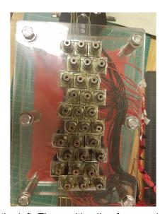
Wire the solenoids according to the diagram on the left. The positive line from each solenoid connects to the vertical screw terminals of the GuitarBot in these positions. Combine the grounds into one wire and attach it to the Screw Shield according to the wiring diagram.
