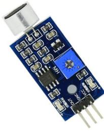
**Instructions:** the sound intensity of the surrounding environment can be detected. When the sound of the external environment fails to reach the set threshold, OUT outputs a high level; when the sound intensity of the environment reaches the set threshold, module OUT outputs a low level. The blue digital potentiometer on the module can be used to adjust the sensitivity.
