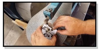
The bits are separated and cleaned ready for painting
