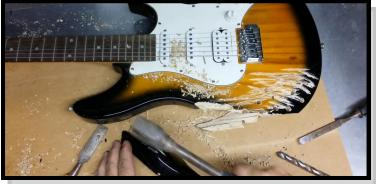
Drill larger holes to start and splinter to surface further
