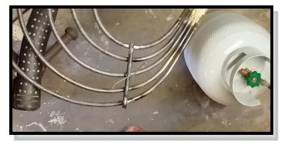
Clamp and wire the parts to make sure they can't move around while you are joining them
