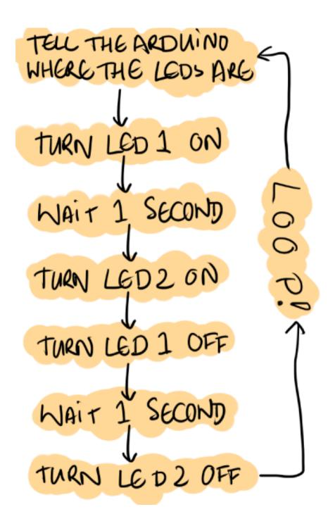
Another example of this process is shown here, where two lights are connected to different pins so that they can be controlled separately to each other. In this example, one LED is connected to pin 9 and the other to pin 10 on the arduino board.
