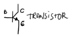
**Transistors** are tiny chips that can work as **amplifiers** or switches. They can either be used to amplify the strength of a weaker electrical signal and make it stronger. This was first used in hearing aids where a tiny microphone would pick up the sound around it, send that to a transistor as an electrical signal where it would be amplified and then fed back out through a louder speaker.
