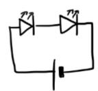
you would need 6V to run the circuit. Since the LEDs are in series (one after the other), they need twice as much power to run.
