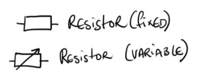
is a resistor with a varying resistance.
