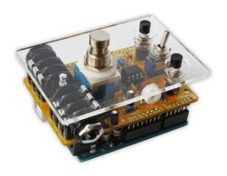
Finally the plastic cover can be placed, it is kept in placed by the foot-switch nut and plastic washer, simple and neat.
