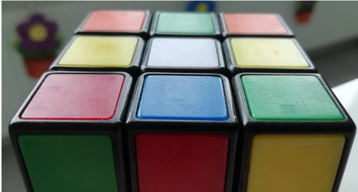
Cube with in-moulded coloured facelet, that I've made matt with sandpaper (grit 1000)
