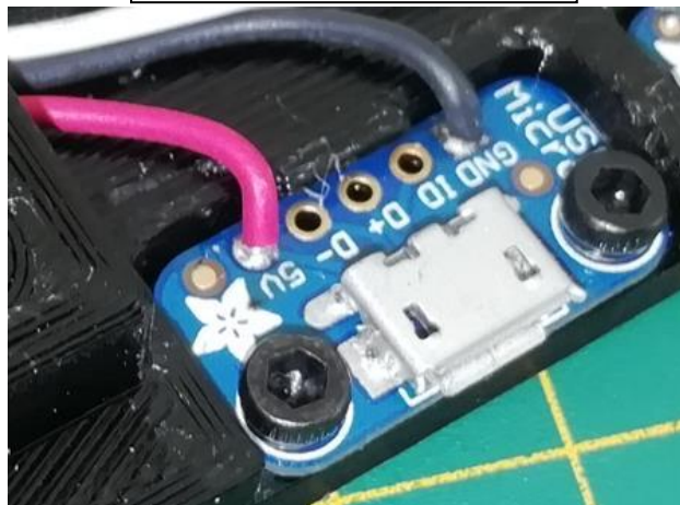
microUSB breakout board: Wire soldering orientation
